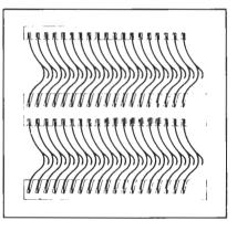
Type T 120/2 resp. T 125/2 Mist eliminator unit similar to T 120 or T 125 but of doubled layer construction used for high face velocities in all kinds of chemical plants.
