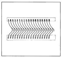
Type T 120, T 125, resp. T 130 Mist eliminator unit with a pitch of 20 mm (T 120) or 25 mm (T 125) or 30 mm (T 130) used when favourable flow conditions and low liquid load prevail.
