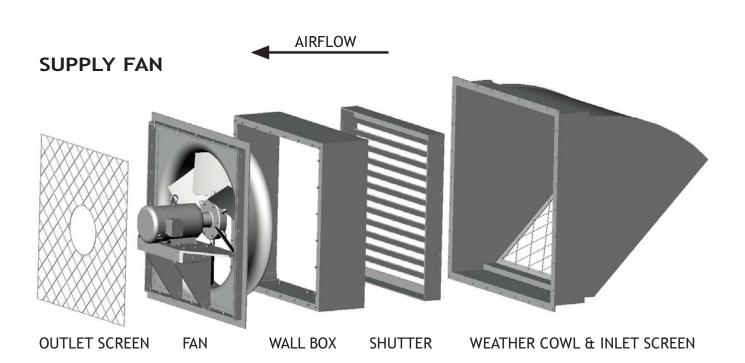
WALL BOX an FRP box to contain fan, shutter and outlet screen. To be mounted in the wall opening. SHUTTER counterbalanced PVC blades. Easily opened with minimal pressure losses. SCREENS PVC/PP/PE, to protect access to inlet or outlet. Stainless steel screens are also available. WEATHER COWL for supply fan configuration.
