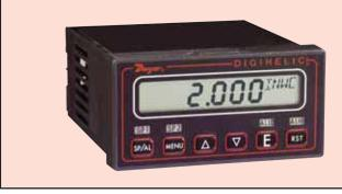
The Series DH Digihelic® Differential Pressure **Controller** is a 3-in-1 instrument possessing a digital display gage, control relay switches, and a transmitter with current output. Combining these three features allows the reduction of several instruments with one product, saving inventory, installation time and money. The Digihelic® controller is the ideal instrument for pressure, velocity and flow applications, achieving a 0.5% full scale accuracy on ranges from 5 to 100 in. w.c.
