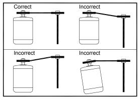
Figure 9 - Pulley Alignment
