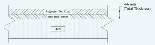
M.K. Plastics Polyester Powder Coating System is fully cured at 390°F, and a final pencil hardness of 2H+, has high humidity resistance (Humidity ASTM-D2247 = 4,000 hrs), and the coating also exceeds 4,000 hrs ASTM-B117 Salt Spray Test.
