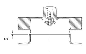
Fig. 4 - Wheel/Inlet Clearance
