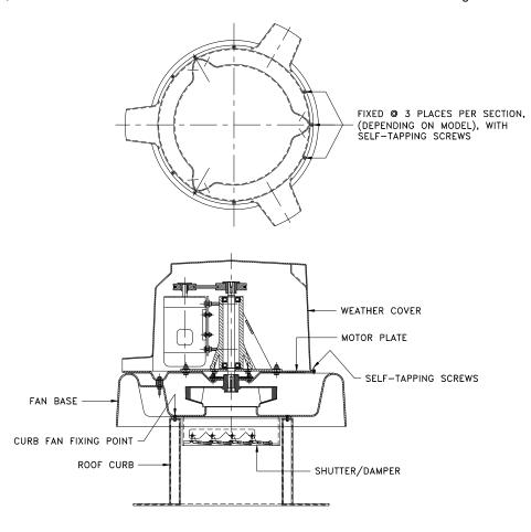
Fig. 2 – Roof Curb Mounted
