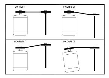
Fig. 6 - Pulley Alignment
