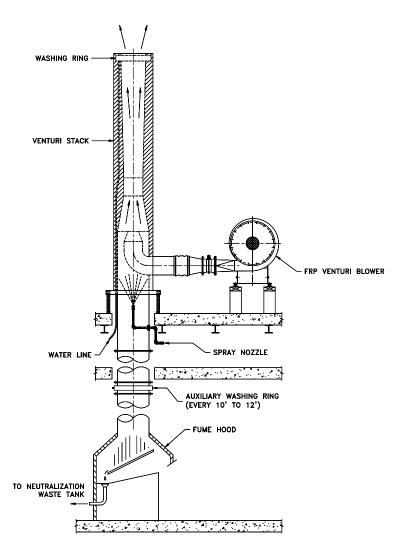
Fig. 1 – MVT Venturi Layout
