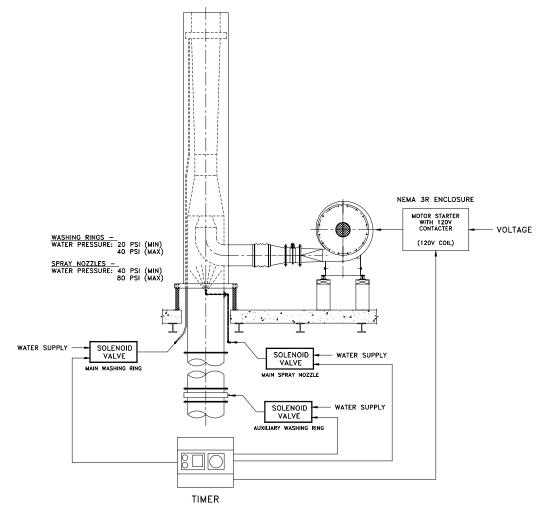
Fig. 4 – Washing Schematic (Typ.)
