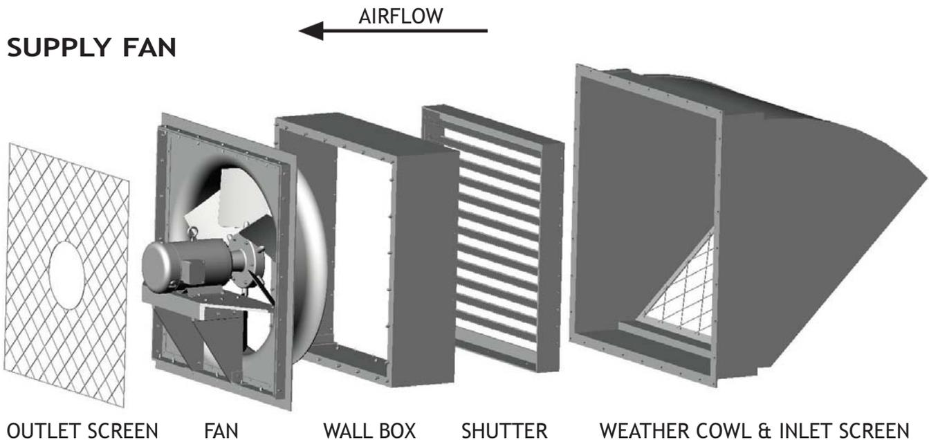
**WALL BOX** an FRP box to contain fan, shutter and outlet screen. To be mounted in the wall opening.
